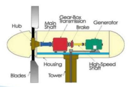
→ Rotor:- The portion of the wind turbine that collects energy from the wind is called the rotor. The rotor usually consists of two or more wooden, fiberglass or metal blades (new design) which rotate about an axis (horizontal or vertical) at a rate determined by the wind speed and the shape of the blades. The blades are attached to the hub, which in turn is attached to the main shaft.
